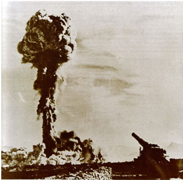
The Grable test resulted in the successful detonation of a 15 kiloton shell (warhead W9) at a range of 7 miles. This was the first and only nuclear shell to be fired from a cannon.
